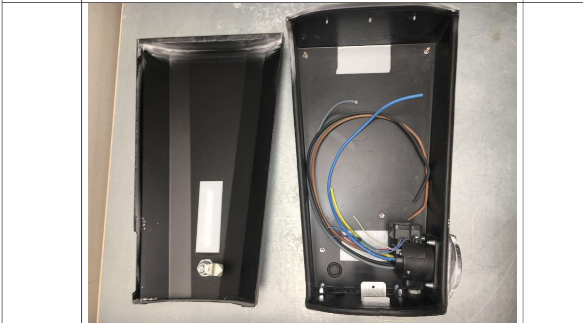
Picture 4 No trace of dust after the dust test.
