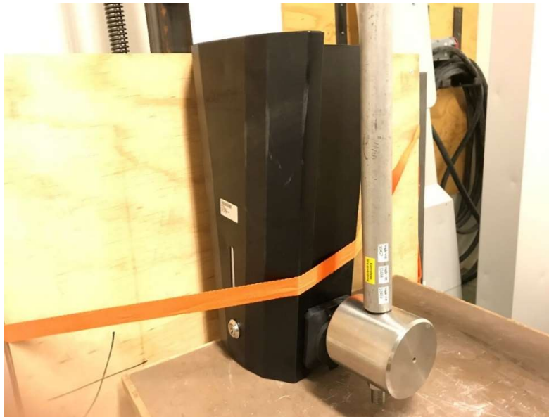
Picture 2: 1 of 5 impact point on exposed surface (right).
