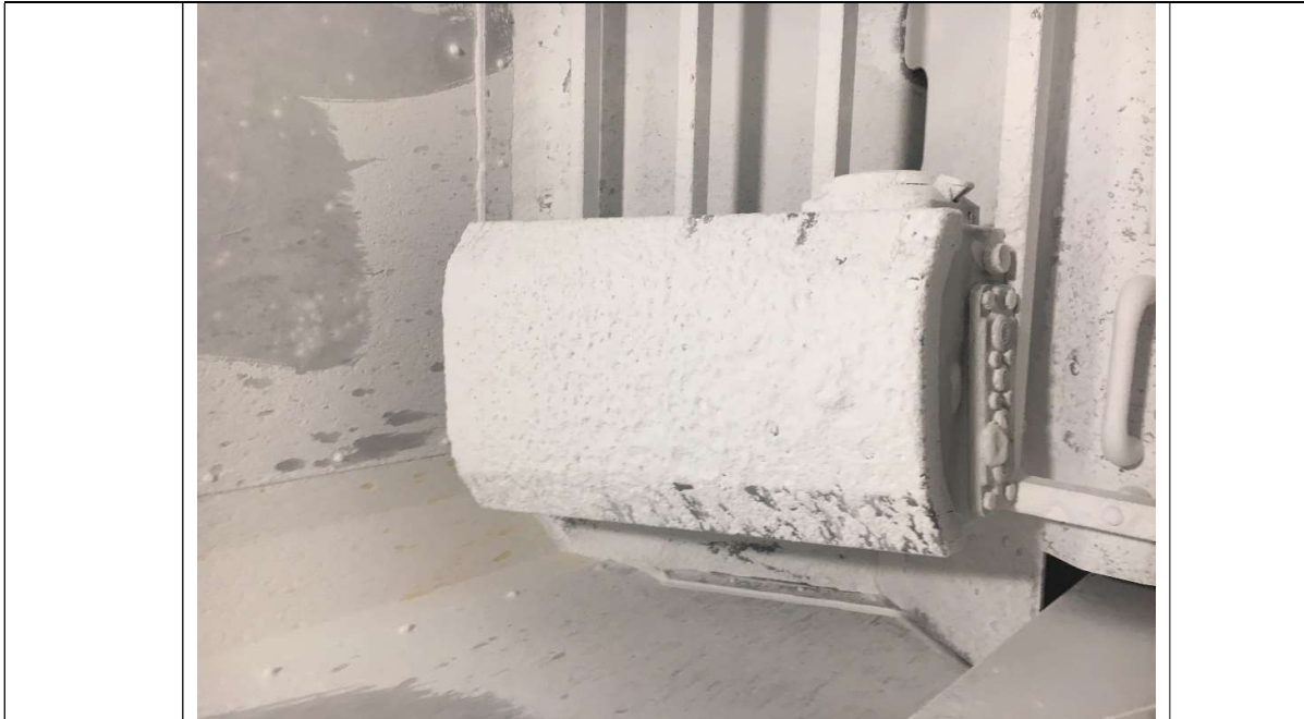
Picture 3 Dust chamber with no pressure difference.
