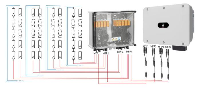
With this installation variant, 8 cables are saved due to the early bundling of the strings in the combiner box. This is about 80m less cable in a typical residential building. In addition, only 8 Y-cables need to be purchased. This saves time and material in the end.
