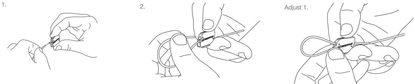
Ensure a minimum 75 mm of tail wire exit the hanger.
