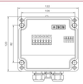
Remark: The ETS-05-A2-E has two rotary switches for the temperature set point. Range is between 0°C and 49°C
