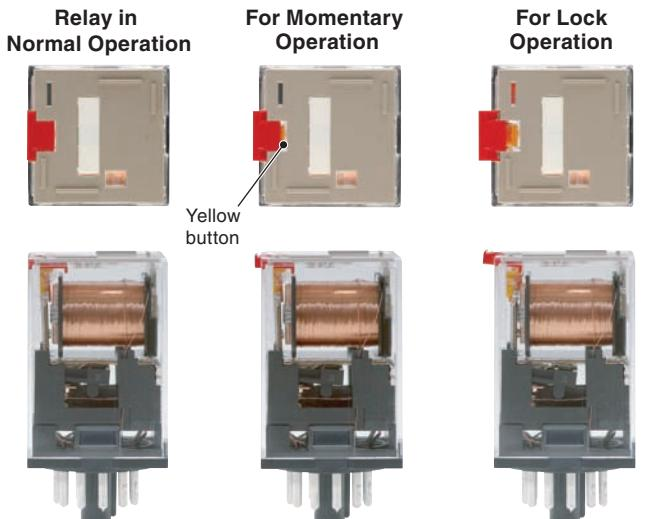
Slide the latching lever to the first position, then press the yellow button with an insulated tool to operate the contact.
