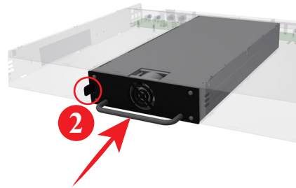
Figure 4.23 Push firmly until the ratchet lock the module
