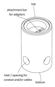
Unimi-1Base<sup>TM</sup> foundation is designed as a hardware agnostic attachment point for electric vehicle (EV) chargers. The foundation is dug into the ground to such depth that the top of the foundation is flush with ground or relevant paving material. The EV charger is attached to the Unimi-1Base<sup>TM</sup> foundation using an adapter. If no EV charger is immediately attached, a separate lid (manhole cover) is used to cover the foundation opening.
