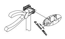
Step 4: Cut the excess wires off.
