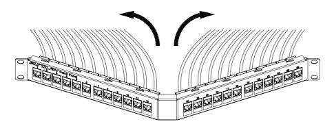
STEP 3: Recommended cable routing in fan direction.
