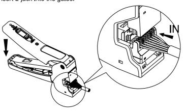
STEP 4: Press L-tool to terminate L-jack and cut extra wires.
