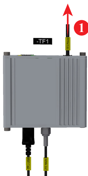
Figure 4.7 Removing power cable from 4G router
