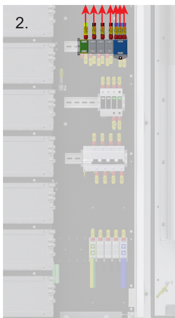
Figure 4.4 Disconnecting cables from terminals -X2
