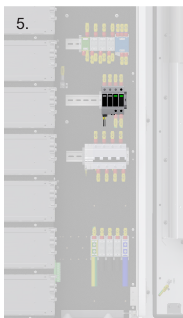
Figure 4.7 Disconnecting wires from SPD -FA1
