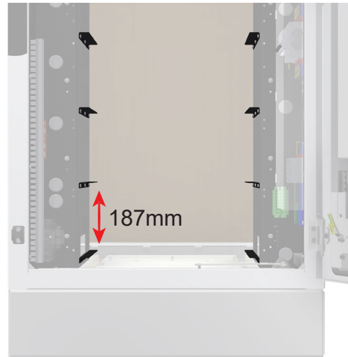
Figure 4.32 4U battery option
