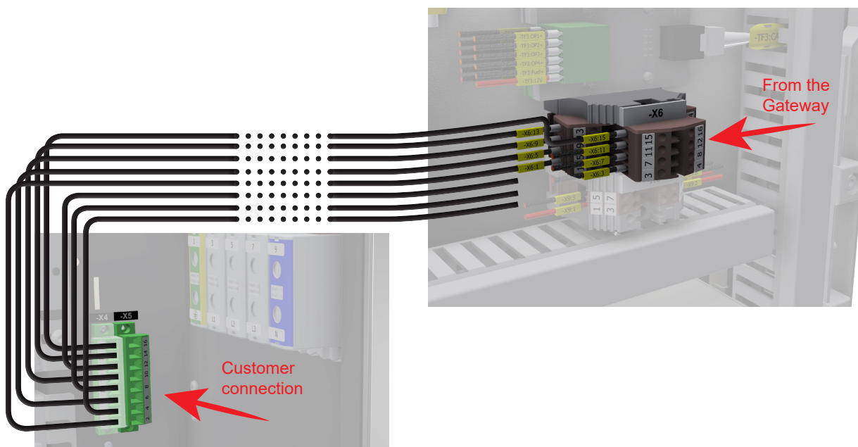
Figure 4.22 Customer spare terminals connection
