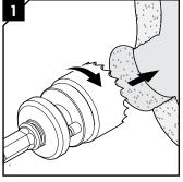
Use a hole saw with the appropriate diameter.
