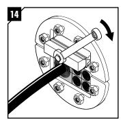
Use the Roxtec pre-compression tool to make room for the final module row.
