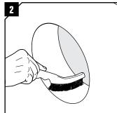
Remove any dirt from the sleeve/ hole.
