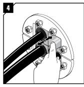
Lubricate the inside surfaces all around with Roxtec Lubricant, especially into the corners. Continue the reinstallation on page 3, step 10.
