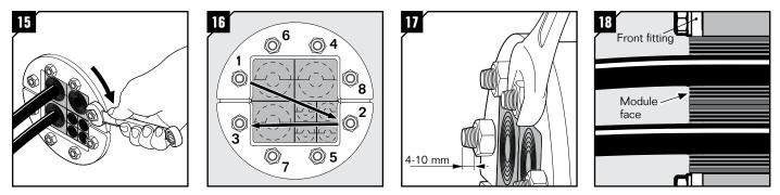
Tighten the nuts crosswise until 4-10 mm thread is visible or the module faces are flush with the front fittings of the R frame.
