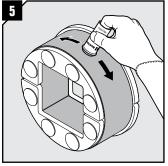
Lubricate the frame sparsely on the outside with Roxtec Lubricant if needed.
