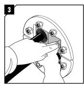
Make sure that the inside surfaces of the packing space are free from dirt or dust.
