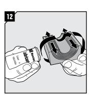
Pull the pipes/cables through. Cables shall go straight through the seal.
