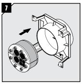
The seal must always be installed in the correct end of the knock-out sleeve.
