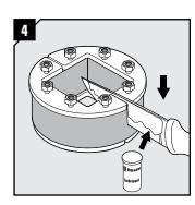
If pipes/cables are pre-routed, the frame can be cut open with a sharp lubricated tool.
