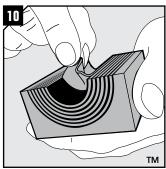
Adapt modules to cables/pipes by peeling off layers. Achieve a 0-1.0 mm gap between the two halves when held against the cable/pipe. The halves may not differ by more than one layer. The last layer must not be removed.
