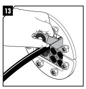
Insert the modules and cables/ pipes according to your installation plan (transit plan). Begin with the smallest modules.
