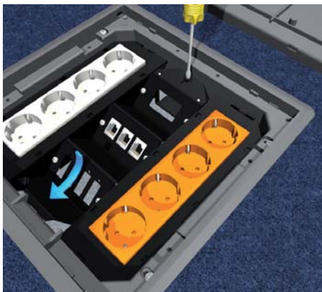
4 | Assembly of data-device carriers Insert device carrier into the installation unit's lock-in leads and secure the latch on the opposite side with a screw into the lock-in.
