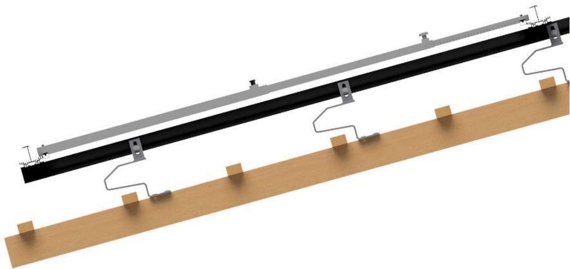
Figure 151: Positioned assembly jig
