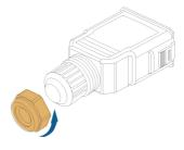
step 2 (Optional) Remove the inner sealing ring if the cable diameter is 19 mm–25 mm. Otherwise skip this step.
