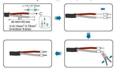
step 6 Plug the wires or terminals into the corresponding terminals as shown in the following figure.
