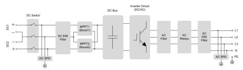
figure 2-4 Circuit Diagram (SG5.0RT for example)
