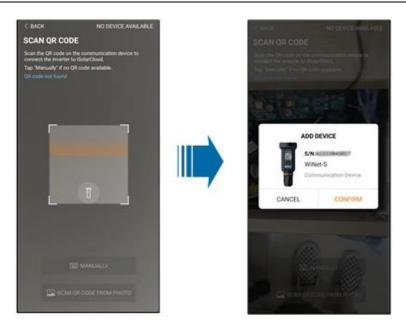
step 6 After a device is bound, tap **Device** and **Commissioning** to go to corresponding interface.
