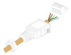
step 5 Remove 80 mm–90 mm of the cable jacket and 12 mm of the wire insulation.
