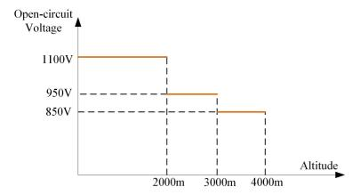
figure 5-4 Open-circuit Voltage Derating Curve
