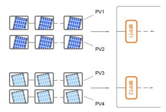
figure 5-3 PV Input Configuration (SG20RT for example)
