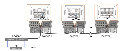
figure 5-6 Multi-inverter Connection
