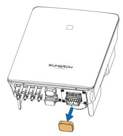
step 3 Lift the locking part upwards and insert the AC connector into the **AC** terminal on the bottom side of the inverter. Then press the locking part and secure it with the screw.
