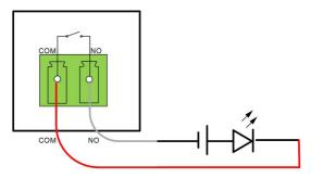
figure 5-9 DO Normal Open Connect
