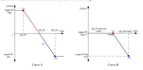
figure 7-20 Reactive Power Regulation Curve in Q(P) Mode
