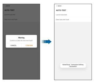
figure 7-25 Clear Auto-test Fault
