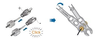
step 5 Check for polarity correctness.
