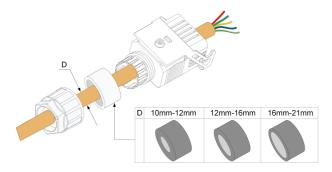
step 4 Remove 45 mm of the cable jacket and 12 mm-16 mm of the wire insulation.
