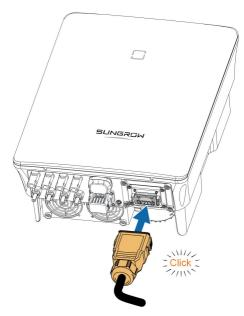
step 4 (Optional) Secure the AC connector, as shown in the figure below.
