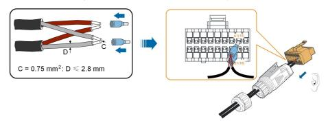
figure 5-8 RS485 daisy chain connection
