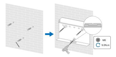
step 3 Lift the inverter and slide it down along the wall-mounting bracket to make sure they match perfectly. Use the fastener set to lock the device.
