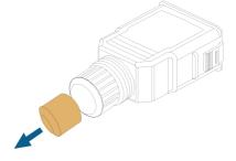
step 3 Take out the screw-type terminal plug from the housing.
