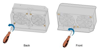
step 7 Use a soft brush or vacuum cleaner to clean the fan. If you need to replace the fan, use a screwdriver to unscrew the screw at the fan bracket and remove the fan.
