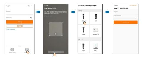
figure 7-2 WLAN Local Access
