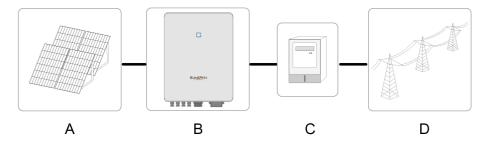
figure 2-1 Inverter Application in PV Power System
