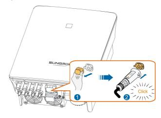
step 7 Slightly shake it by hand to determine whether it is installed firmly.
