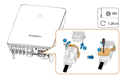
step 4 Connect the PE wire to ground and the phase lines and the "N" line to AC circuit breaker.
