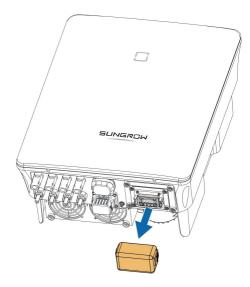
step 3 Insert the AC connector into the **AC** terminal on the bottom of the inverter until there is an audible sound.
