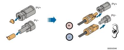
step 4 Seal the unused PV terminals with the terminal caps.
