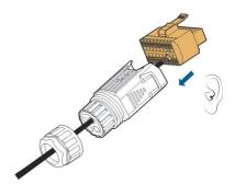
step 8 **For RS485 daisy chain:** Crimp two wires A to a two-wire core end terminal and two wires B to another terminal. Plug the terminals to A1 and B1 respectively.
