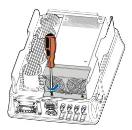
step 5 Lift the fan bracket upwards, press down the protrusion on the fan power plug connector and pull it outwards, and remove the fan bracket.
