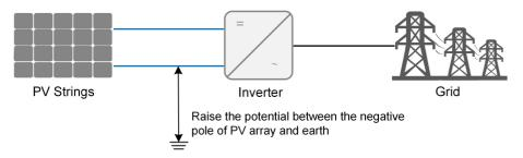
For negative voltage scheme, after the PID function is enabled, the voltage to ground of all PV strings is lower than 0, and therefore the PV string-to-ground voltage is a negative value.
