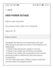
figure 7-9 Detailed Fault Alarm Information
