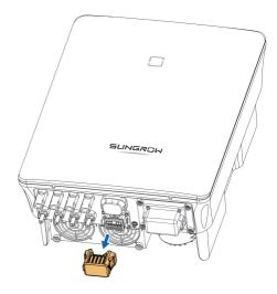
step 2 Insert the COM connector into **COM2** terminal on the bottom of the inverter until there is an audible click.
