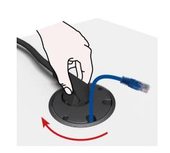
Rotate plug clockwise to reattach.
