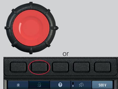
**WARNING :** When the insulation test is locked on, the instrument does not discharge the circuit or asset at the end of a test. The circuit and test-leads remain live and hazardous. Ensure that you discharge the circuit safely before touching any connections.
