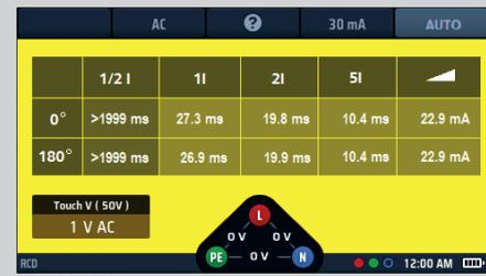
Fig 44: AUTO RCD test result progress
