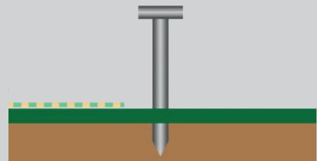
4. Drive a test stake into the ground at least 2 m away from the electrode you are testing.
