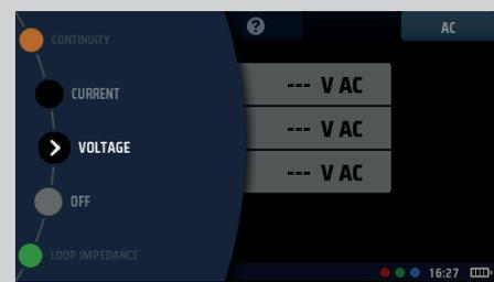
2. For a two-wire test, plug your test-leads into the green and red sockets as indicated in the INFO bar..
