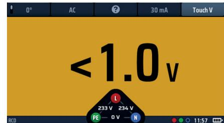
**NOTE :** Connection can be made at the end of the circuit, in the distribution board or on the RCD
