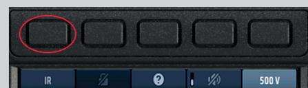
4. Press Hot key 5 until the test voltage you want is shown below it.
