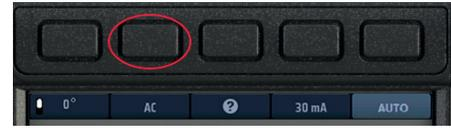
5. Repeatedly press Hot key 4 until the current rating of the RCD you are testing is shown.
