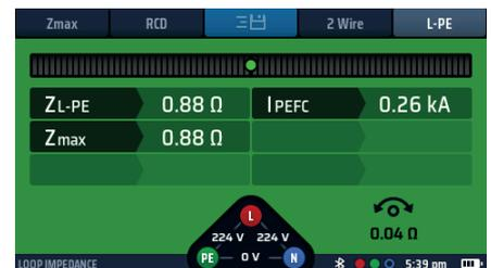
11. Reconnect the instrument at the next point where you want to measure Z<sub>max</sub>. If AUTO START is enabled in settings press the test button BEFORE connecting the test-leads.
