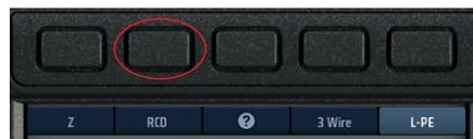
5. Repeatedly press Hot key 4 to select either 2-wire or 3-wire testing. The example (right) uses 3-wire connection.
