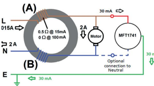
Fig 41: Simplified RCD circuit
