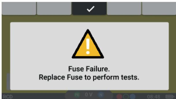
**Fig 59:** Fuse fail warning
