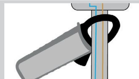
4. You do not need to press the test button. The test starts automatically as soon as you have positioned the clamp.
