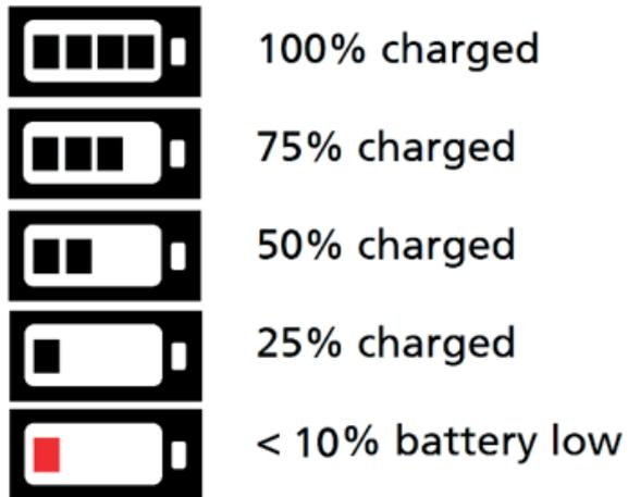
When the battery is very low the last battery cell will turn red. Tests can be prevented in this state. The battery needs to be recharged.
