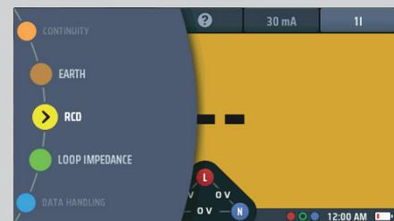
2. For Type AC and A RCDs you can use two-wire testing. Plug your L (red) test-lead into the red socket and your PE (green) test-lead into the green socket.
