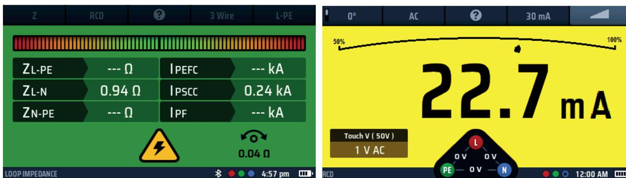
Fig 26: Live test voltage warning - Loop testing and RCD testing examples
