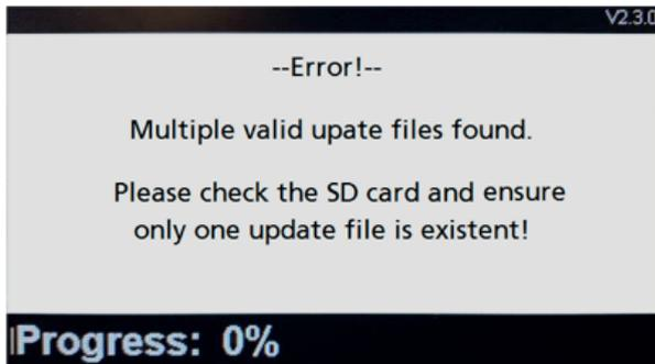
**Fig 57:** Example Error screen
