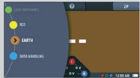
2. Press Hot key 1 to select a test voltage of 25 V or 50 V.
