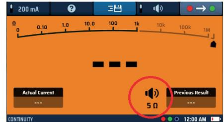
**Fig 17:** Continuity buzzer and threshold
