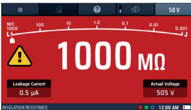
Fig 20: Insulation test in progress
