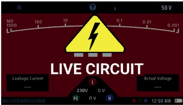
Fig 21: Live circuit warning screen
