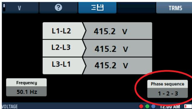
**Fig 34: Voltage phase rotation**
