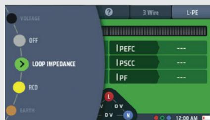
2. Plug your red L test-lead into the red socket and your green PE test-lead into the green socket.
