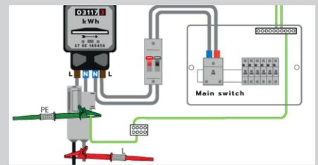
The example here shows connection for an L-PE measurement.
