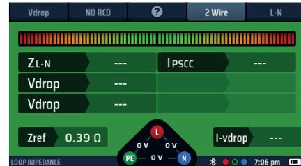
3. Turn the right rotary knob to select Set I-vdrop. Hot key 3 will change to Set I-vdrop for 3 seconds. Press Hot key 3 to accept.
