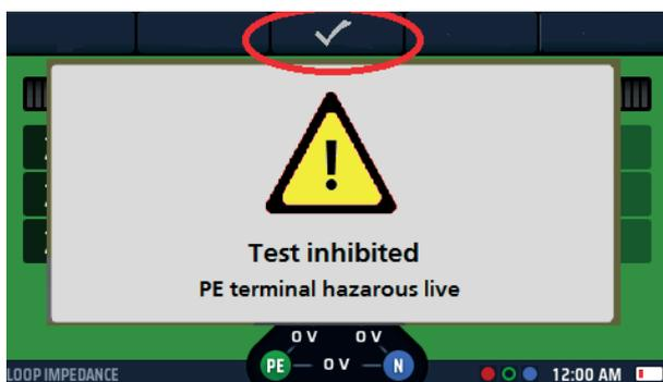
**Fig 28:** PE warning non-blocking
