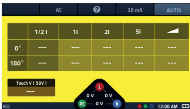
Fig 43: RCD auto test example start screen
