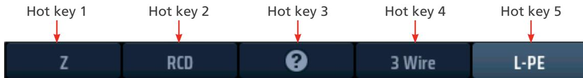
**Fig 48: Loop impedance Hot keys**
