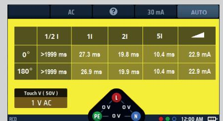
■ If the RCD does not trip the display shows:
