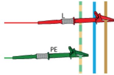
15. After each test, the displays shows the loop impedance (ZL-PE) and the prospective earth-fault current, IPEFC, for the most recent test.
