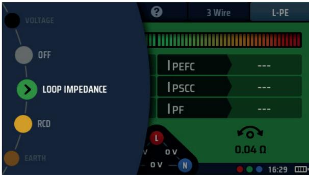
Fig 47: Selecting loop impedance mode
