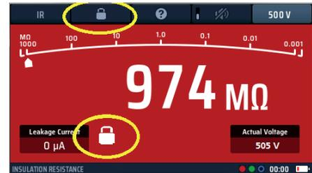
Fig 22: Insulation test lock
