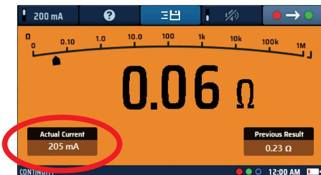
Fig 12: Continuity test current
