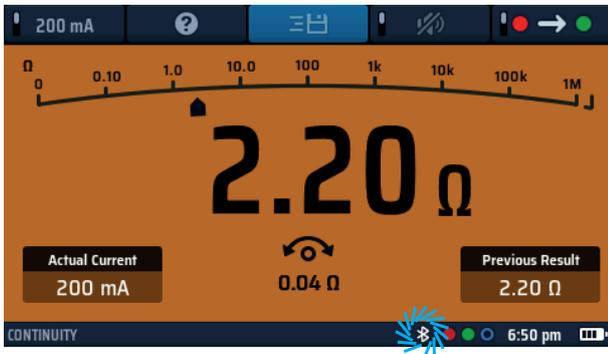
Fig 55: Flashing Bluetooth® icon
