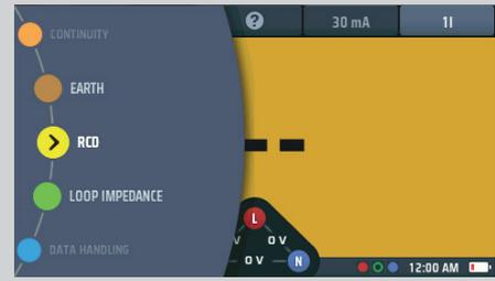
2. For Type AC and A RCDs you can use two-wire testing. Plug your L (red) test-lead into the red socket and your PE (green) test-lead into the green socket.
