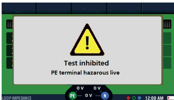
**Fig 27:** PE warning blocking
