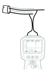
Connect the test lead to the cable under test. Connection may be made to a live power system with a voltage to earth (ground) less than 150 V with an installation (over voltage) category of I V or lower. This means that the instrument may be connected to any to primary supply circuits such as overhead cables. The voltage must be less than 300 V between the terminals and 150 V CAT IV to earth.
