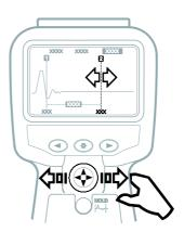
The range is set using the four way switch; press up to increase the range and down to reduce the range.
