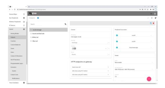
Configure the function of the output as Monostable or Bistable; the differences are described below:
