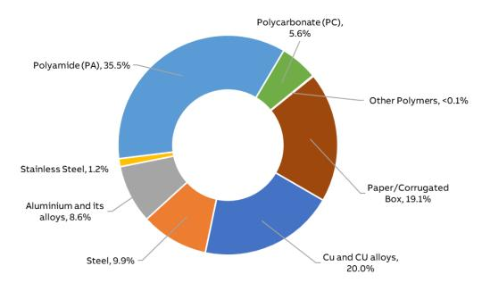
Figure 1: Composition of SLE 1 Fuse Switch Disconnector
