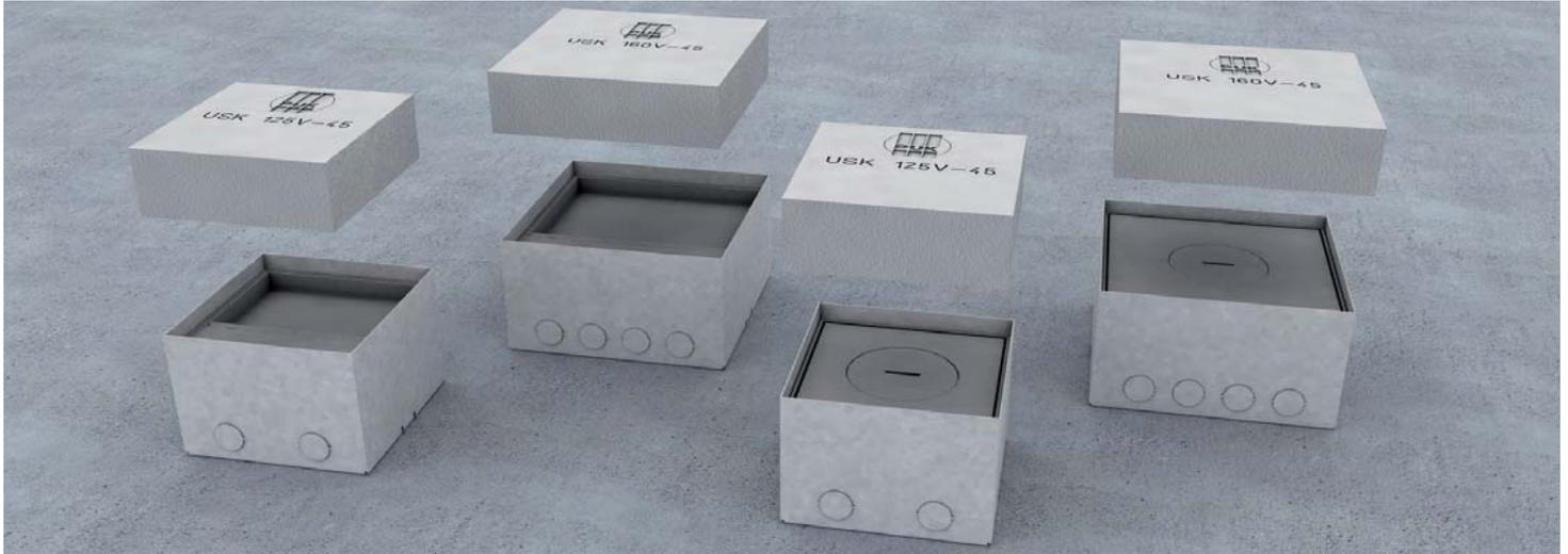
Quadrangular compact single outlet, external dimensions 125 x 125 mm and 160 x 160 mm for installation directly into screed, suitable for dry and wet maintenance rooms. Scope of delivery contains floor box, stainless steel unit and shuttering unit. For parquet and stone floors of 12/22 mm levelling range: 80–125 mm or 90–135 mm.
